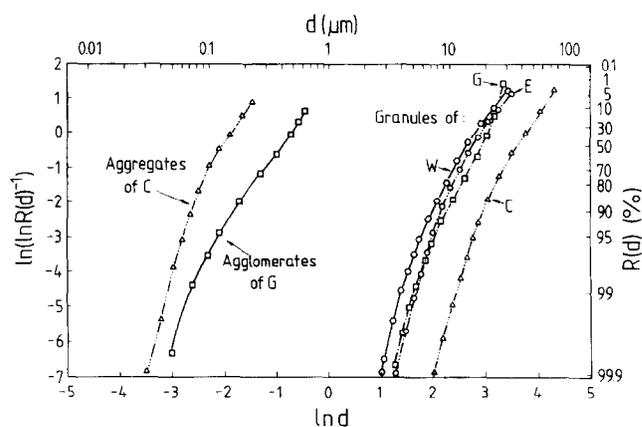
Fig. 2. Agglomerate, aggregate and granule size distribution drawn in the Rosin-Rammler coordinates.
