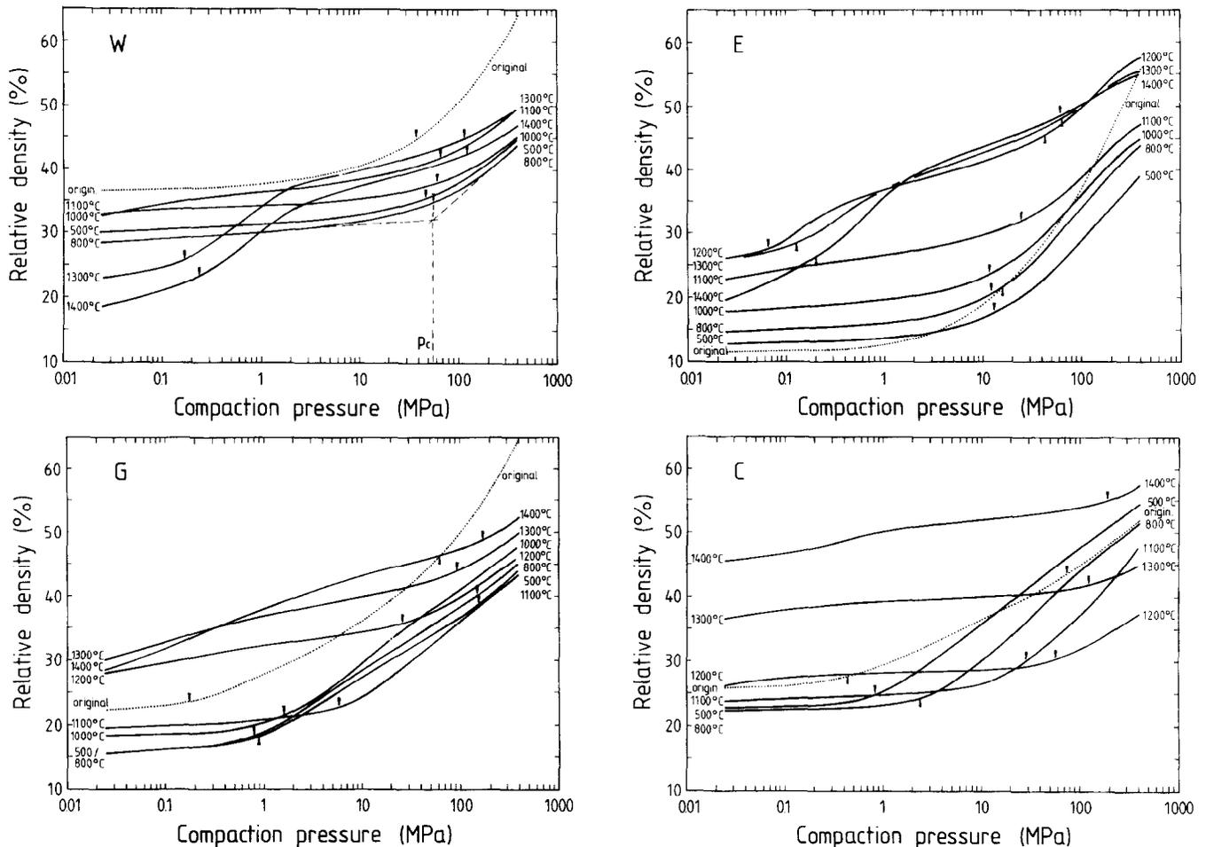
Fig. 9. Compaction curves of the powders: (a) powder W, (b) powder E, (c) powder G, (d) powder C.
