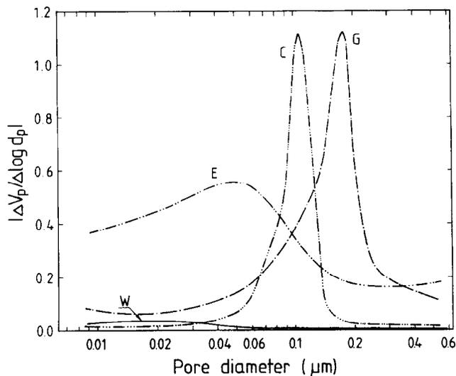
Fig. 4. Pore size distribution curves of the 'as spray dried' granules.
