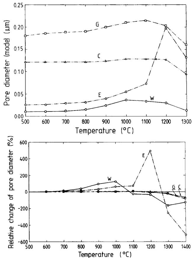
Fig. 6. Modal pore diameter (a) and relative change of modal pore diameter (b) vs temperature of heat treatment.
