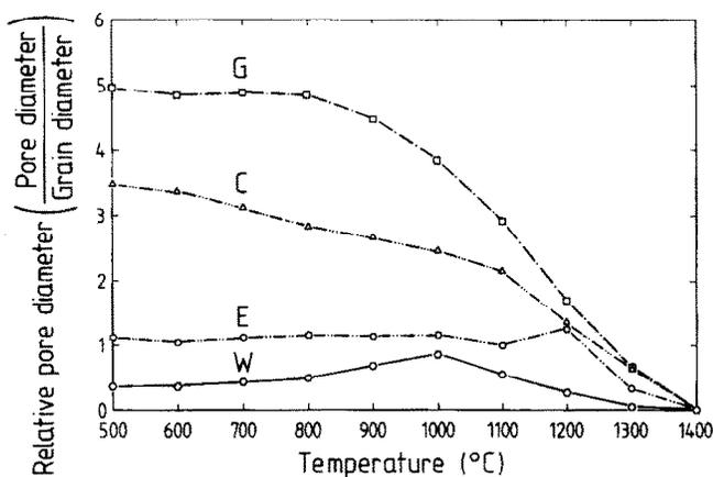
**Fig. 8.** Relative pore diameter vs temperature of heat treatment.
