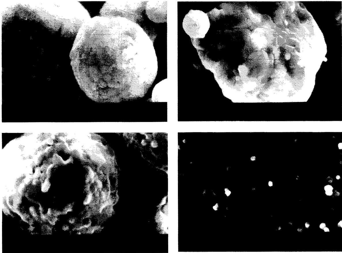
**Fig. 7.** SEM micrographs of the powders sintered at 1400°C: (a) powder W, (b) powder E, (c) powder G, (d) powder C.
