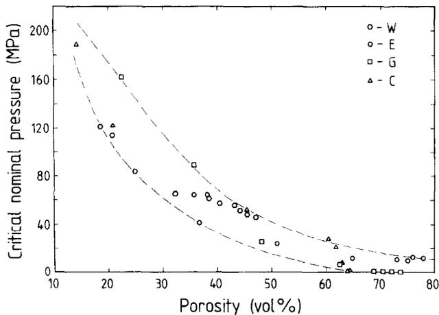
Fig. 10. Critical nominal pressure vs porosity of the granules.
