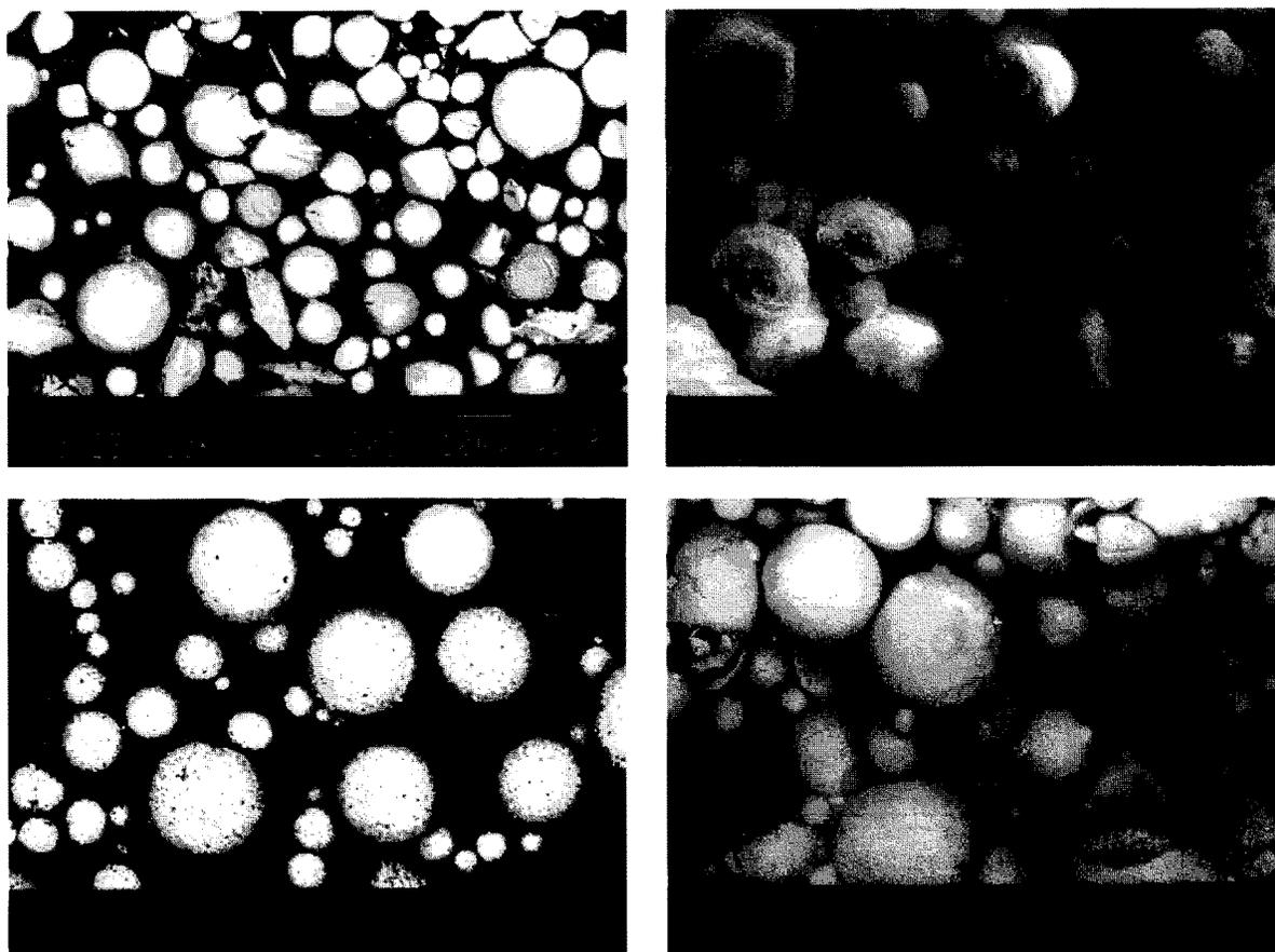
Fig. 3. SEM micrographs of the 'as spray dried' granules: (a) powder W (back scattered), (b) powder E (SEI), (c) powder G (back scattered), (d) powder C (SEI, fractured surface of a compact pressed to  $p_c$ ).
