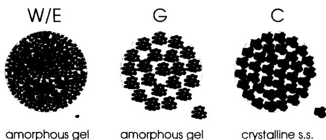
Fig. 1. Scheme of granule microstructures studied. Elementary particles of the powders that were used to form the granules and their crystallinity are indicated.
