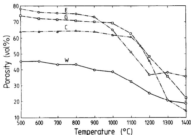
Fig. 5. Porosity of the granules vs temperature of heat treatment.
